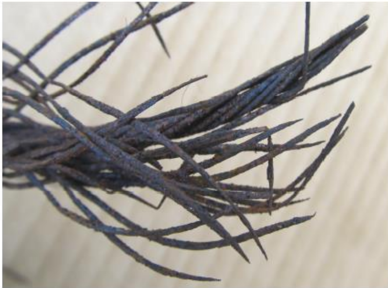
Figure 5. Failure (typical) close up showing severe corrosion of the wires (needle-like points).
