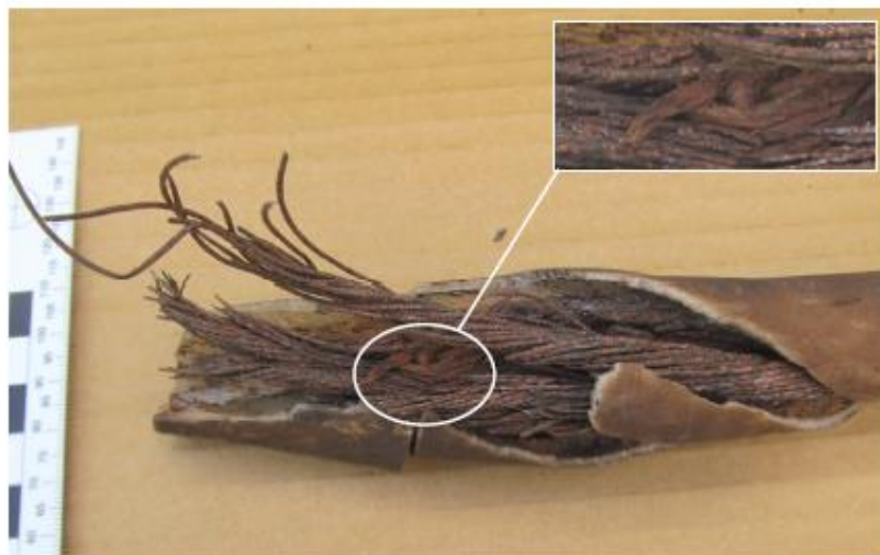
Figure 4. General view of one of the failures. Note the overall corrosion, the fibre rope core (circled and inset) and brittle fracture of the sheath.
