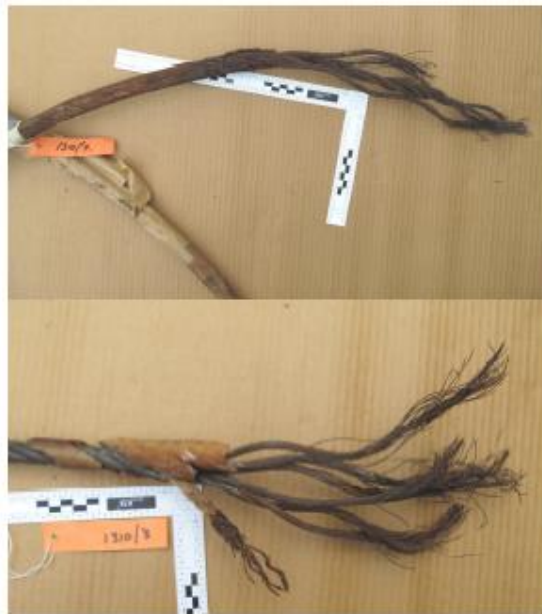
Figure 3. Failed ropes as received.
