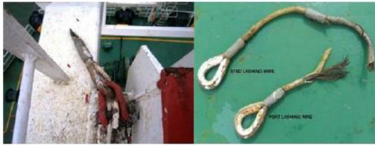
Broken lashing cables, i.e., maintenance wires
