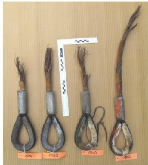
Figure 1. Four portions of the failed wire ropes as received.
