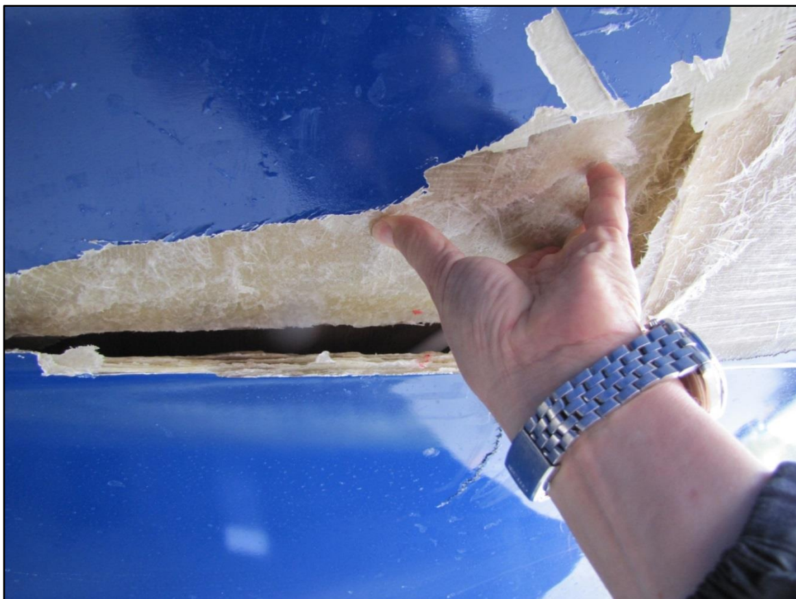
Figure 3 Damage sustained to port underside of bridgedeck
