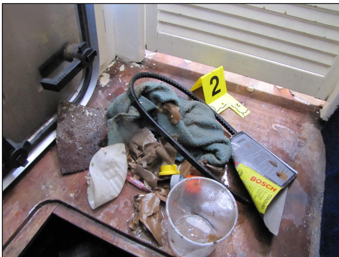
Figure 7 Items recovered from port forward bilge well that were obstructing the bilge suction strainer
