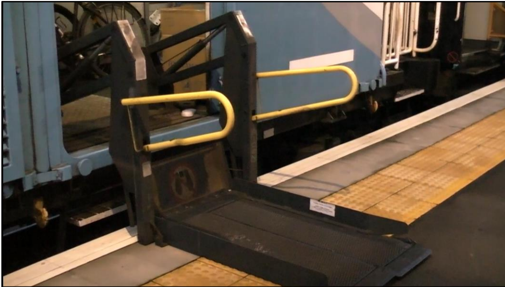
Figure 1 Mobility hoist deployed from the luggage van at Waikanae Station
