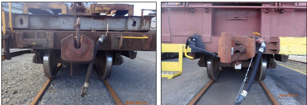
Figure 9 Old standard wagon coupler (left) and new automatic coupler (right)
