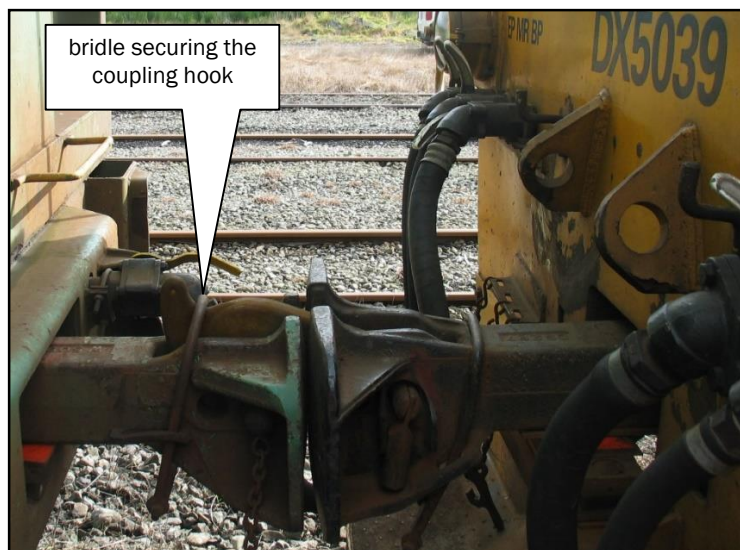
Figure 8 Coupling hook and bridle security arrangements on a standard coupler mechanism
