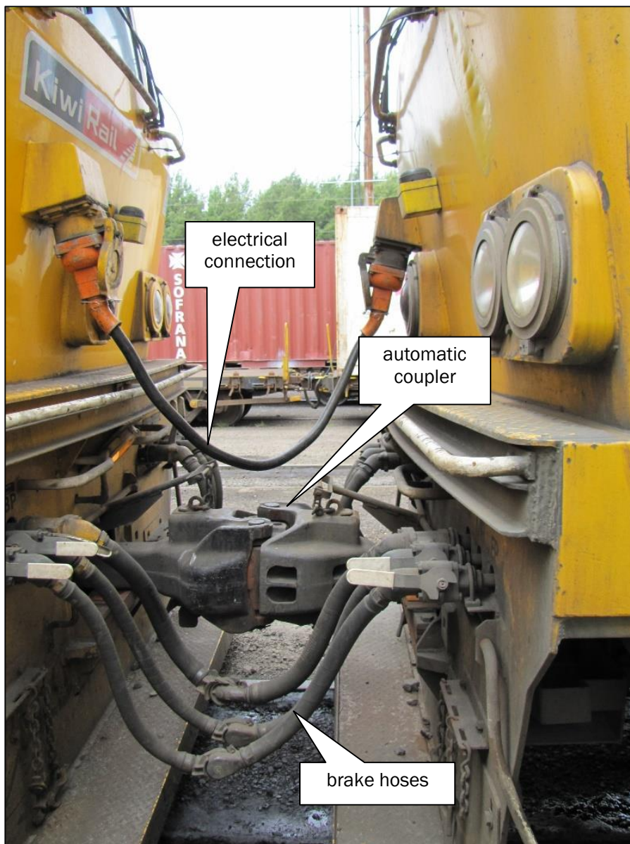
Figure 1 The three components used to join locomotives and wagons to form a train
