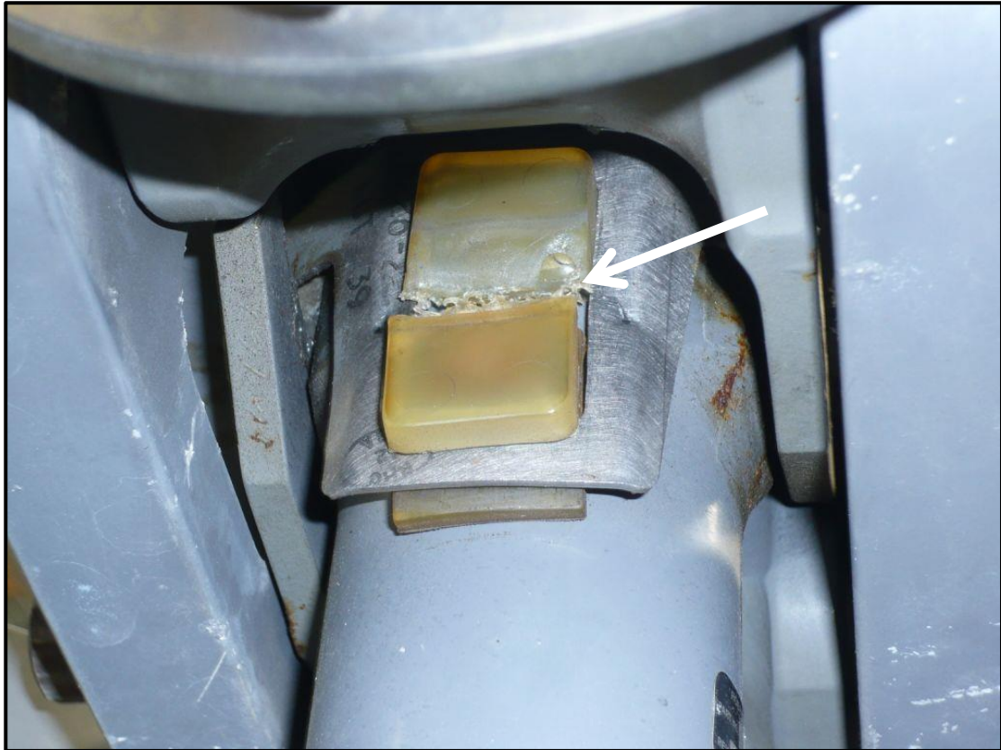
Figure 2 Crushed and split teeter stop
