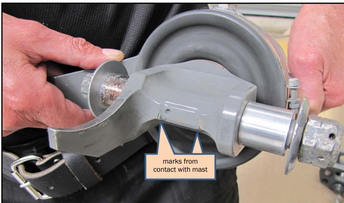
Figure 1 Blade spindle, showing evidence of mast contact
