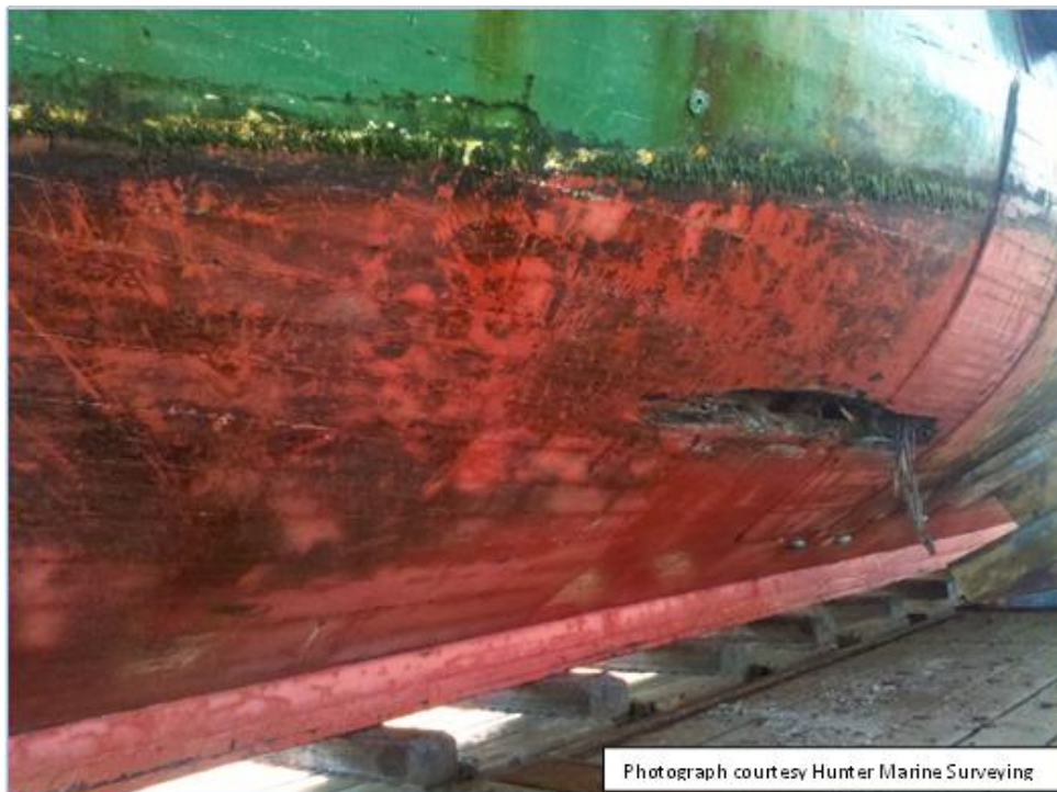
Figure 4 Damage sustained to the port side of the underwater hull of the Torea
