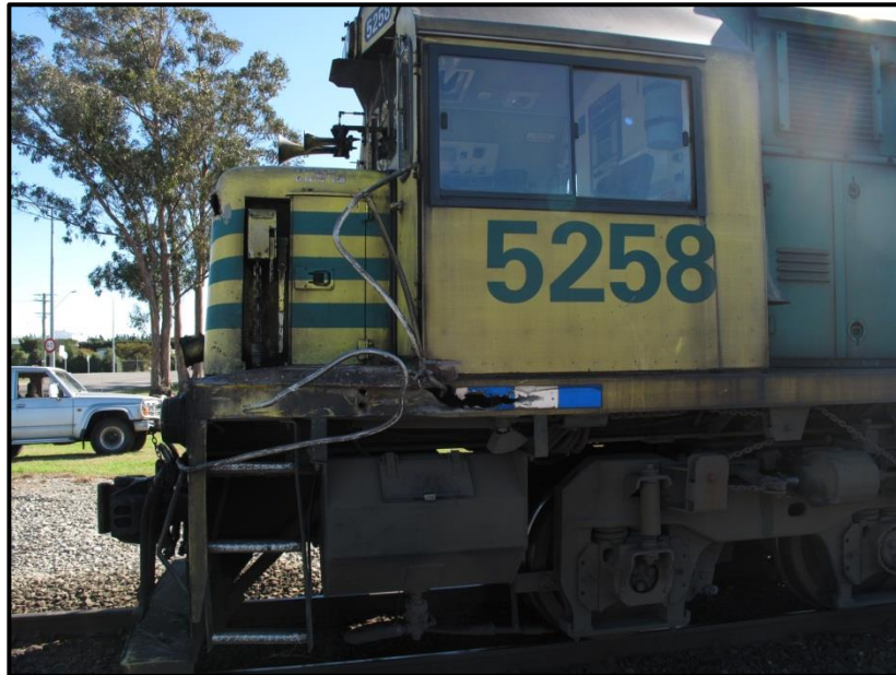
Figure 5 Damage to the locomotive on Train 845
