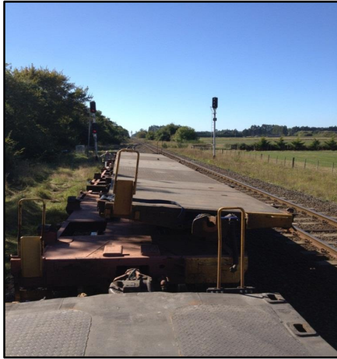
Figure 6 The load overhanging the wagon at Rolleston
