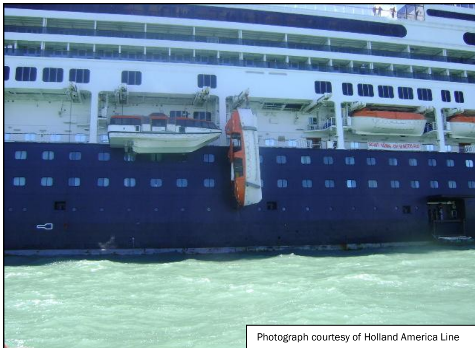
Figure 1 Number 7 lifeboat in vertical position after failure of wire fall
