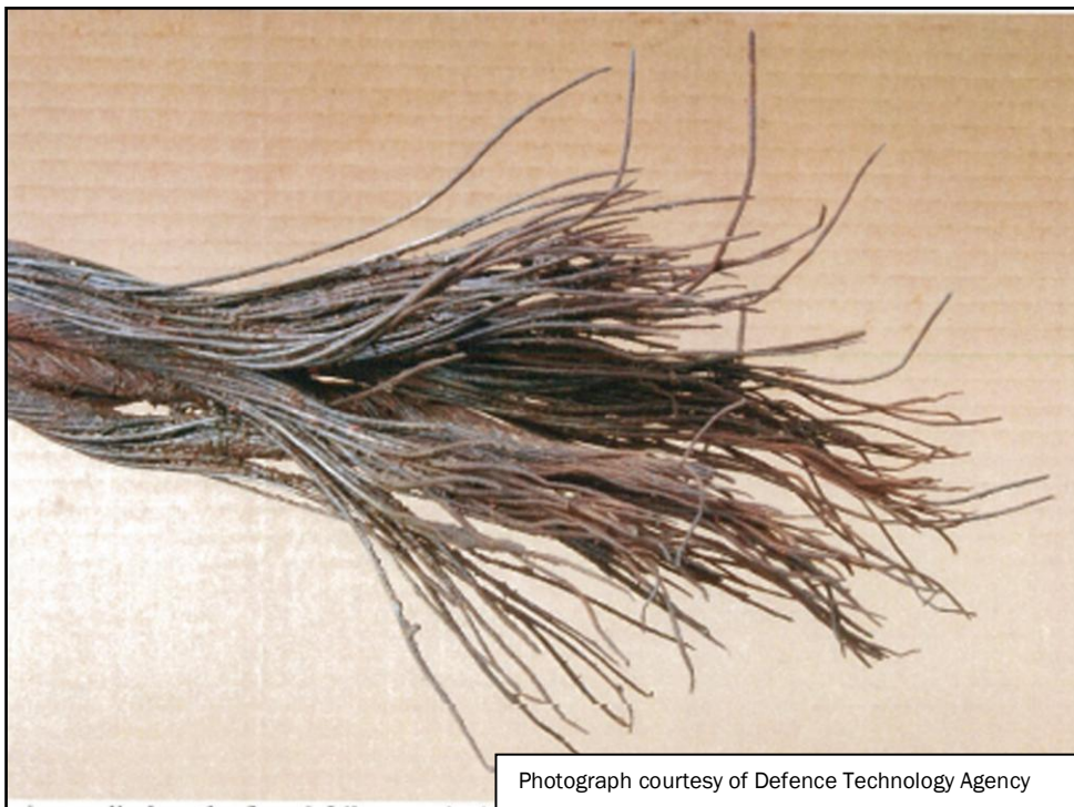
Figure 9 Photograph of the failure point of number 7 lifeboat forward wire fall
