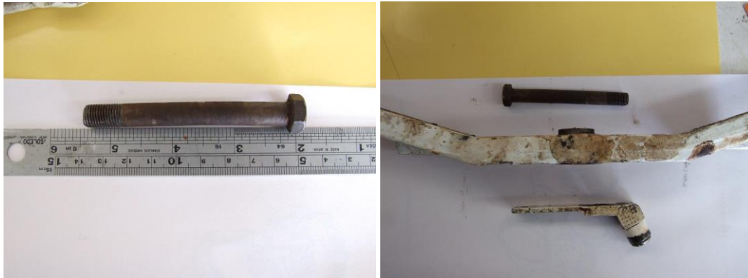
Figure 3 Bent pivot bolt (left), with bell-crank and alignment bracket (right)
