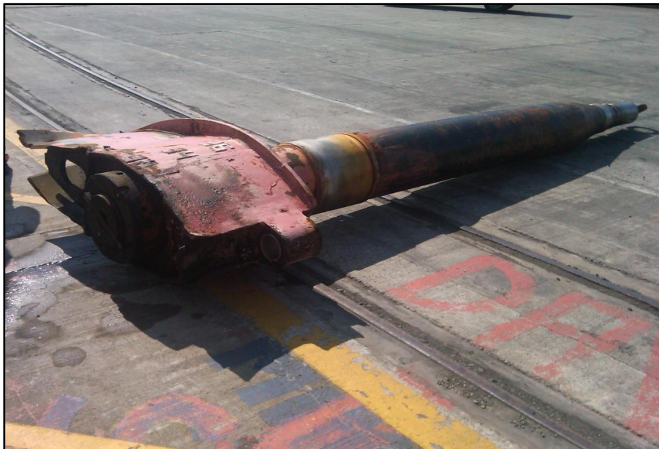
Figure 3 Rudder stock and remaining top part of rudder after removal from ship (Photograph courtesy of Pacifica Transport Group)
