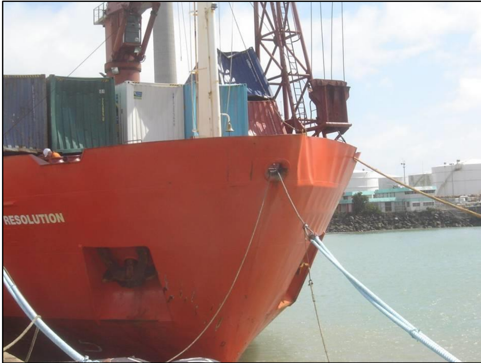
Figure 4 Damage to bulwarks and containers (Photograph courtesy of Pacifica Transport Group)
