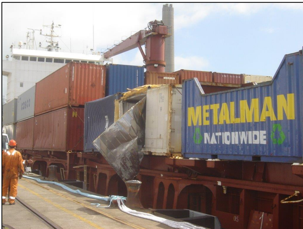
Figure 5 Damage to containers on starboard side (Photograph courtesy of Pacifica Transport Group)
