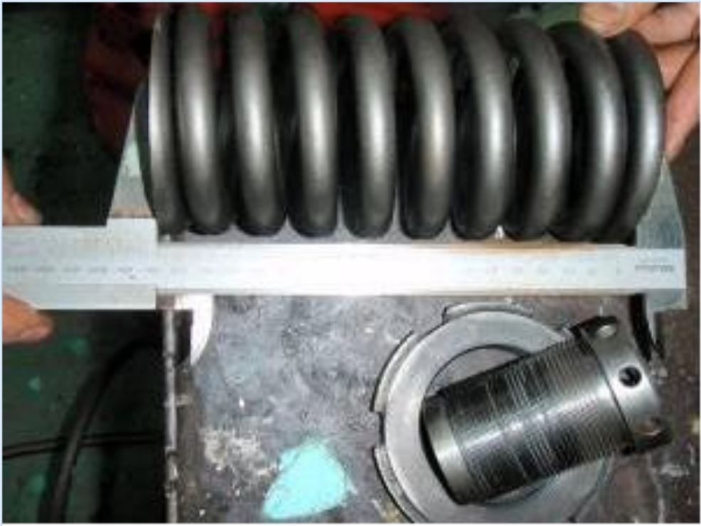
Figure A1-3 Photograph of spring showing condition on disassembly
