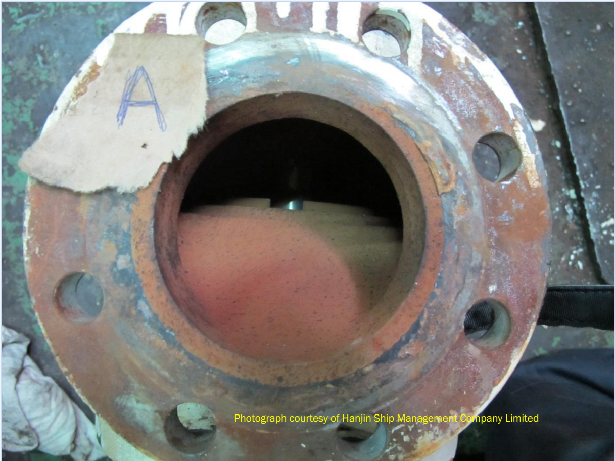
Figure A1-2 View into 3-way valve through bypass inlet showing detritus build-up and “clean” valve stem
