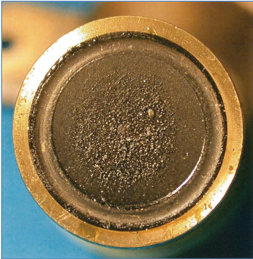
Figure 7 Boost valve seal in end of piston
