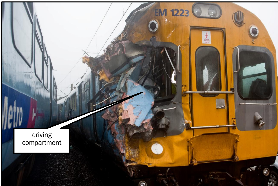
Figure 2 Driving compartment of Train 6247 after impact
