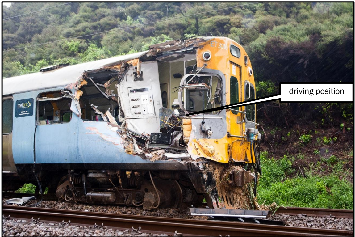
Figure 1 Driving compartment of derailed Train 6250 after being struck by Train 6247
