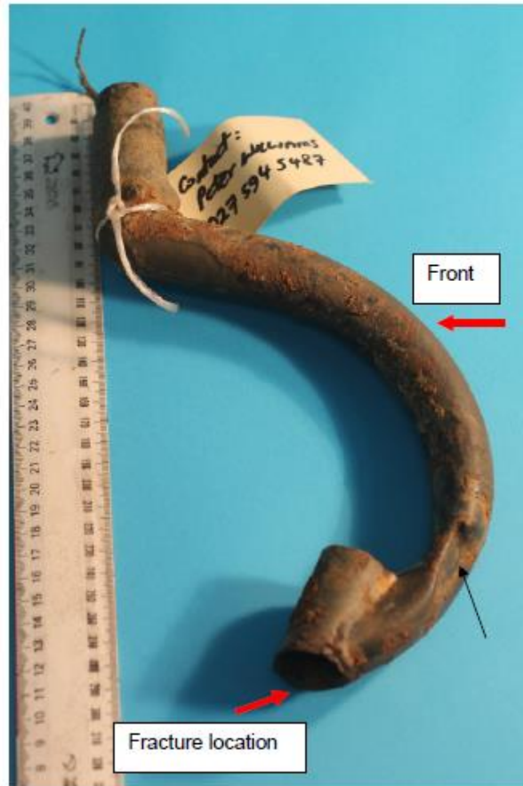
Figure 2: Control Column as supplied. Photomicrograph shows the fractured bottom tube that was welded to the curved tube. The side on the right of the picture was marked F (front). The black arrow shows the probable direction of the impact force which generated damaged found on the curved section of tubing.
