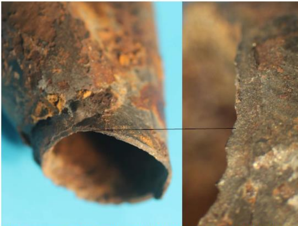
Figure 4: Fracture Surface on bottom tubing, 45 degree shear lip / overload fracture clearly visible.
