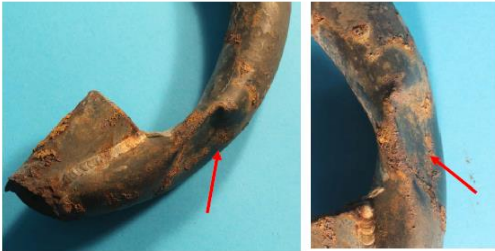
Figure 3: Close up of the indentation / impact damage in the curved tube section. The arrows show the probable direction of the impact force.
