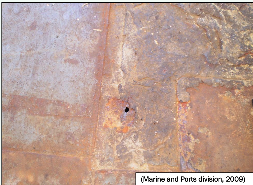
Figure 15 Hole in deck above No 1 void space
