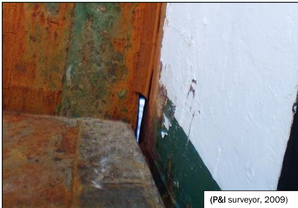
Figure 19 "Gap" beside bow ramp after cement removed
