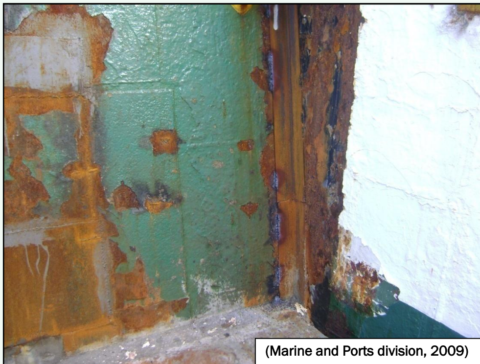
Figure 12 Welded bow ramp with cement covering the hinge
