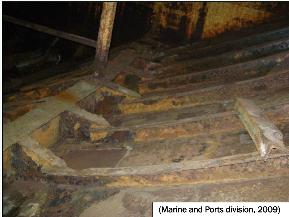
Figure 14 Corroded void space
