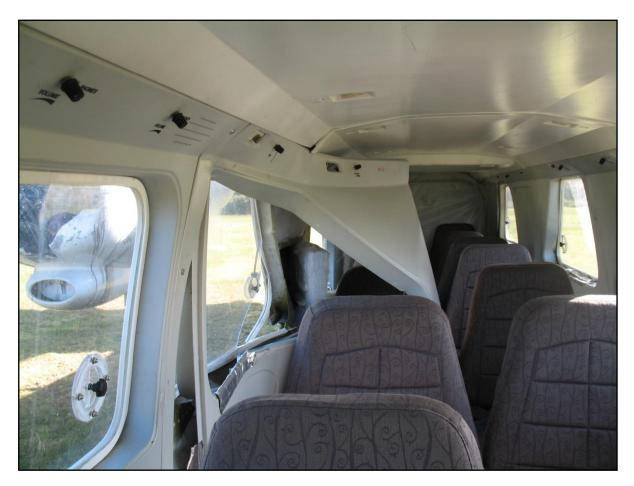
Figure 3 ZK-LOU interior showing cabin lining damage
