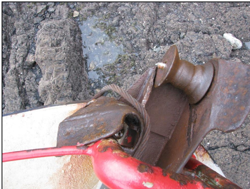
Figure 5 Damaged forward fairlead
