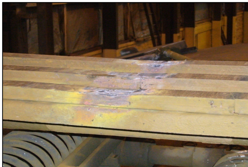
Figure 9 Pantograph damage: Arc damage on contact surface © Transport Accident Investigation Commission
