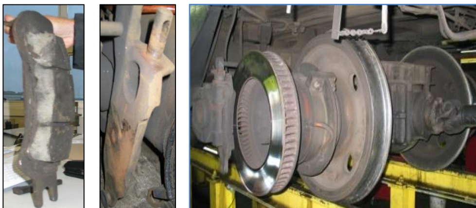
Figure 4 From left to right, brake calliper, backing plate and disc brake arrangement on outside of wheel
