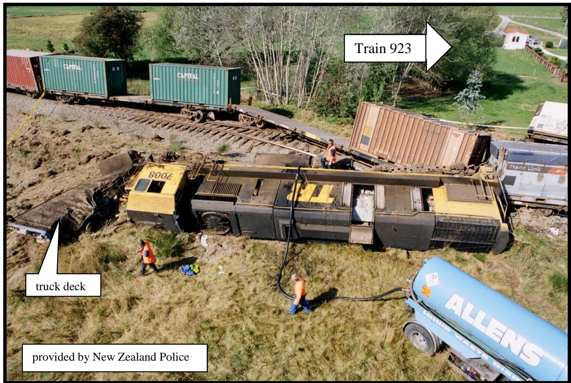
Figure 1 DFT 7008 after the collision
