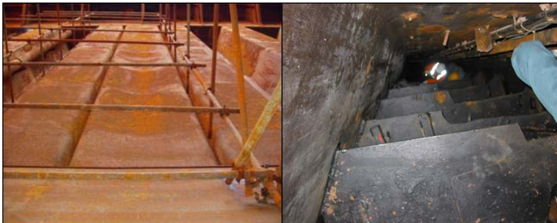
Figure 18 Bulge and temporary repairs to access trunk wall in number 6 hold
