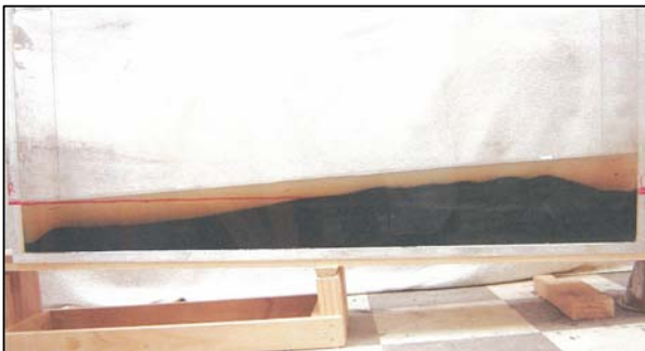
Figure 21 NZ Steel Mining study of cargo shift mechanism
