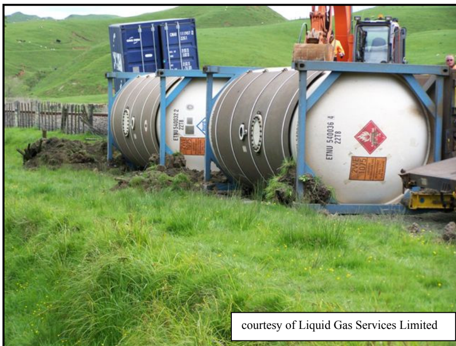
Figure 3 The ISO liquid petroleum gas tanks
