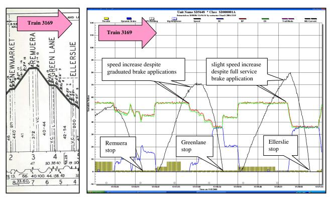
Figure 6 Ellerslie station track alignment/gradient detail (left) and (right) event recorder data from SD5648 (neither graph is to scale) (refer appendix section 6.6 for a larger scale of the event recorder data)
