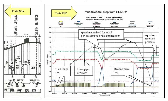
Figure 8 Meadowbank station track alignment/gradient detail (left) and (right) event recorder data from SD5652 (neither graph is to scale) (refer appendix section 6.6 for a larger scale of the event recorder data)
