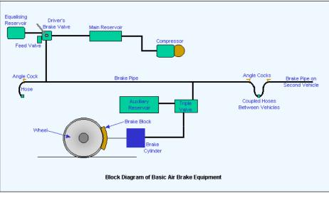
Figure 12 Diagram of a train air brake system (not to scale)
