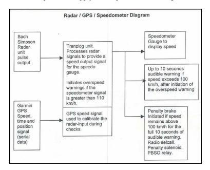
Figure 14 Details of the integrated SD driving trailer speedometer system
