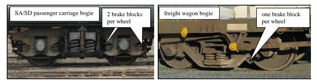
Figure 13 Brake block arrangements
