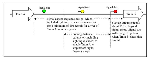
Figure 9 Signal aspect sequence design using 3 signal spacing (not to scale)
