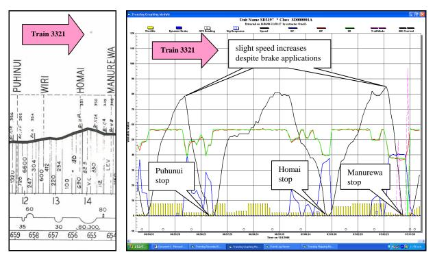
Figure 5 Manurewa station track alignment/gradient detail (left) and (right) event recorder data from SD3197 (neither graph is to scale) (refer appendix section 6.6 for a larger scale of the event recorder data)
