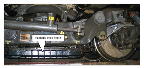
Figure 15 Magnetic track brake on a Norwegian multiple unit vehicle
