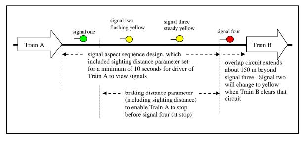
Figure 10 Signal aspect sequence design using 4 signal spacing (not to scale)
