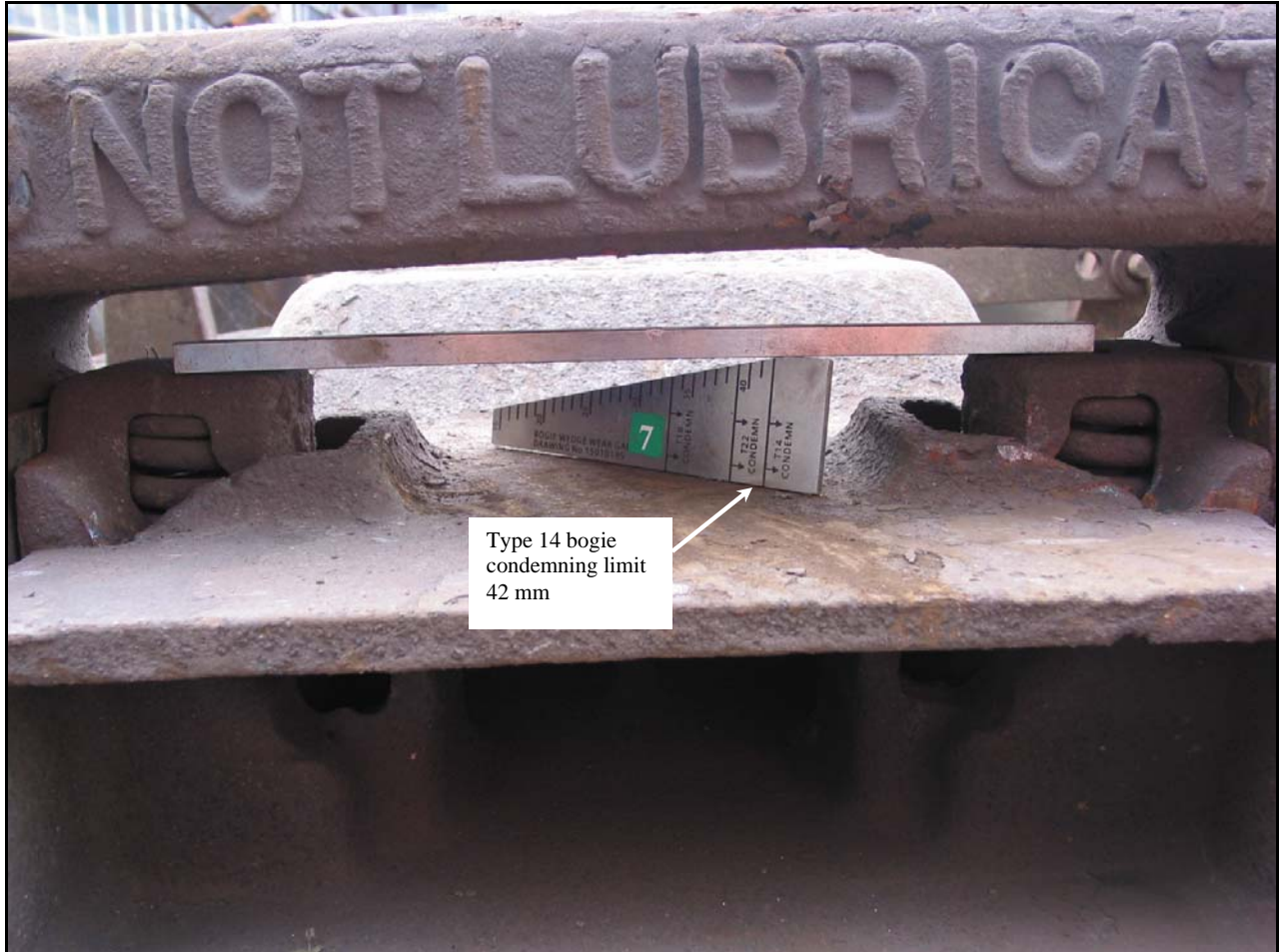
Figure 5 Wedge measurement leading bogie of UK6765
