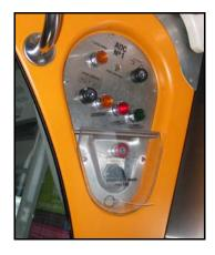
Figure 6 Passenger emergency stop button
