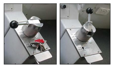
Figure 3 The master controller handle in the throttle 2 setting left; and right, in the application position with the reverser key removed
