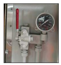
Figure 4 Emergency brake handle on back wall of both cabs
