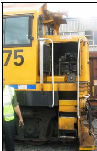
Figure 3 Brake control valve cabinet of DC4375
