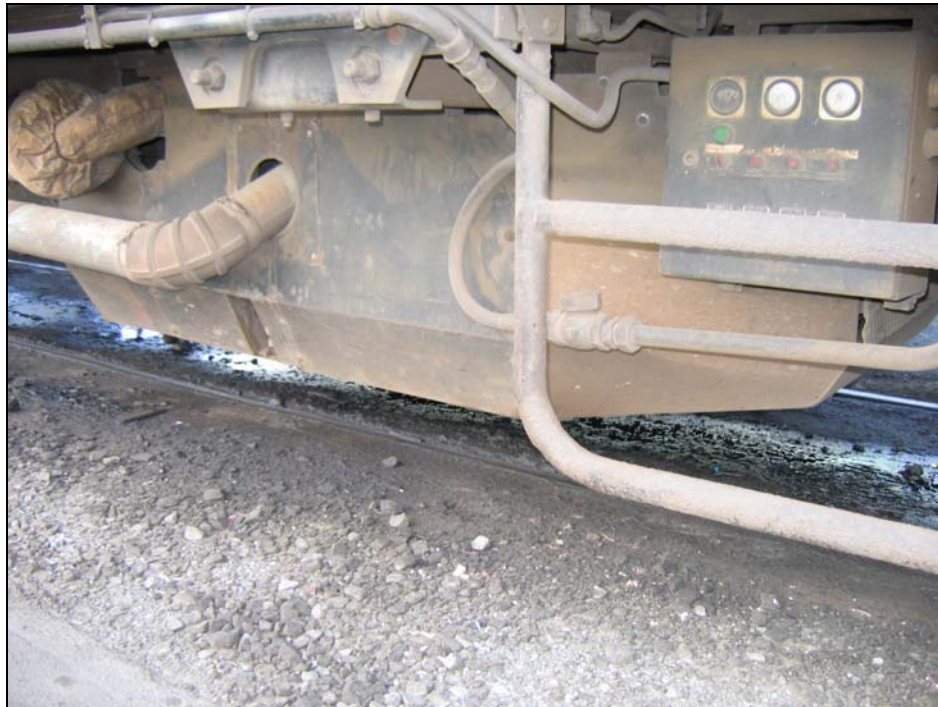
Figure 9 Side shroud on the turbocharger side of ADC857 (courtesy Toll Rail)
