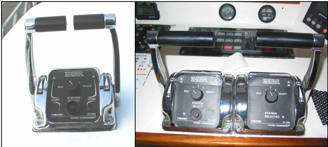
Figure 3 Port bridge wing and wheelhouse engine control stations
