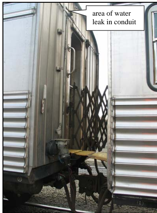
Figure 5 Conduit and jumper plug socket on ADK 687
