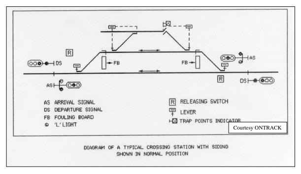
Figure 5 Typical layout of a crossing station in SLAS territory (not to scale)
