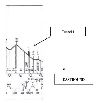
Figure 10 Gradient diagram for Tunnel 1 (courtesy ONTRACK)
