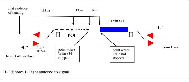
Figure 4 Positions of Trains 841 and 834 after impact (not to scale)
