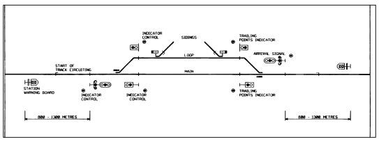
Figure 8 TWC crossing station (courtesy ONTRACK)
