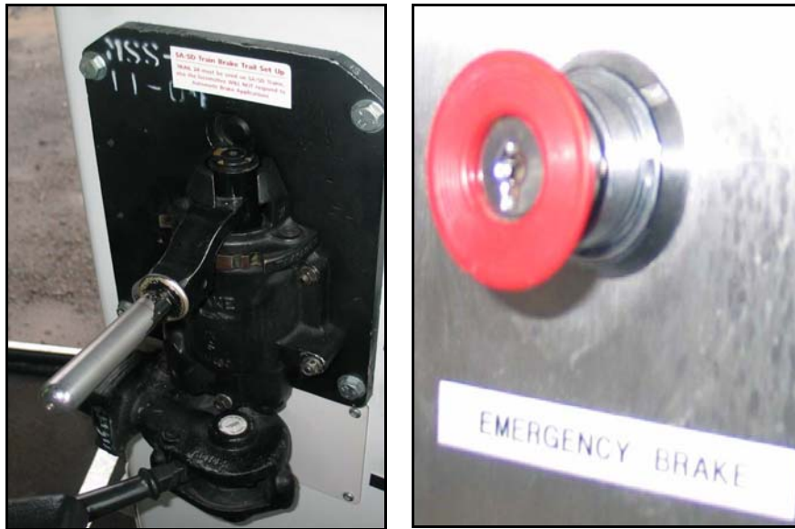
Figure 2 Air brake controls in the driving cab of SD5811
