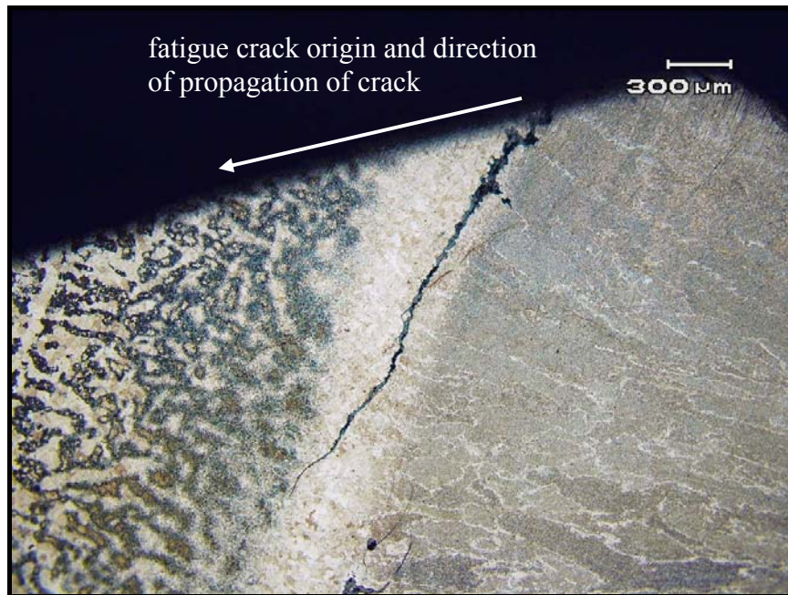
Figure 10 Origin of the fatigue crack in the HAZ
