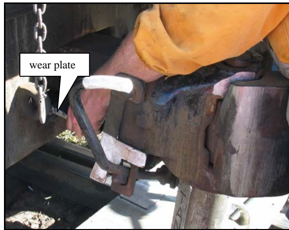
Figure 7 New drawbar wear plate being installed on AG 55
