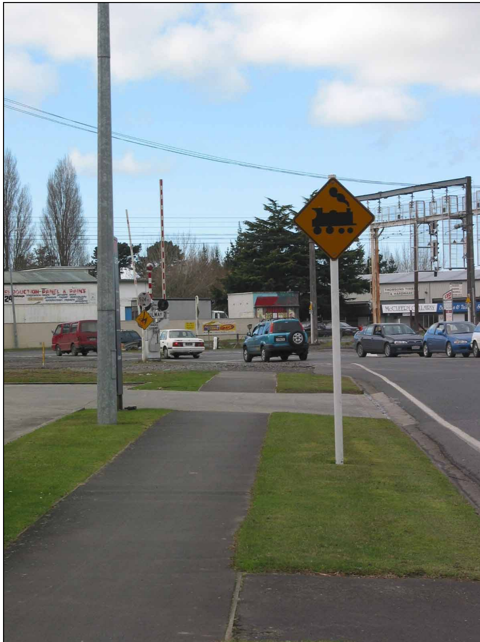
Figure 4 The PW-57 sign on the western side of the crossing
