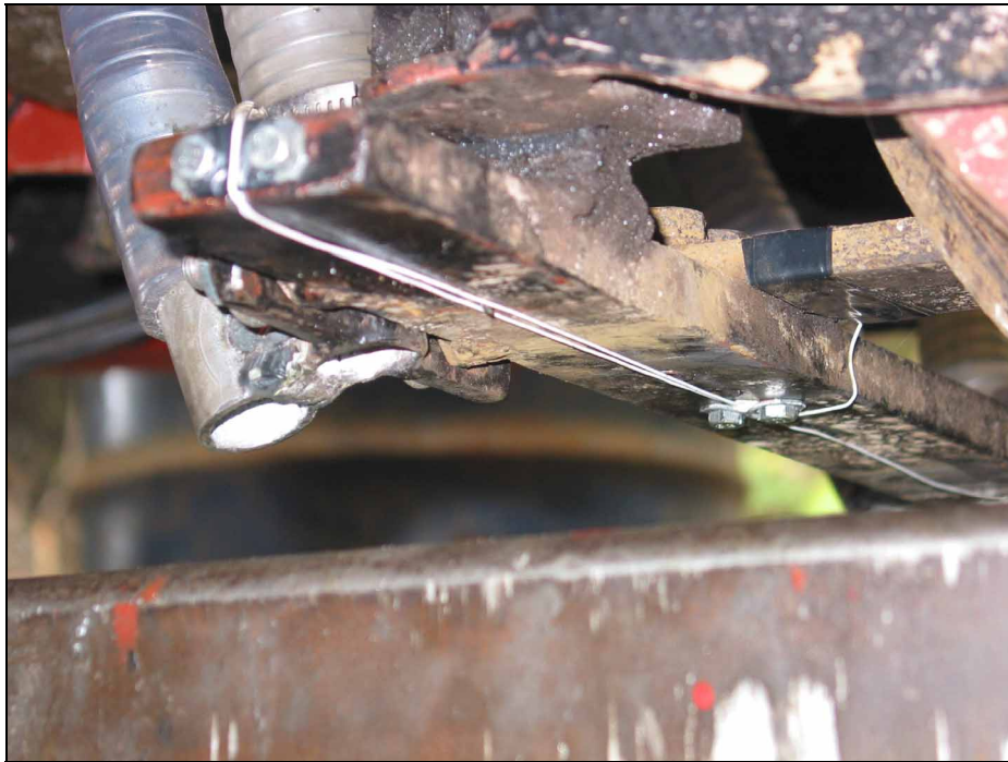
Figure 8 The derailment warning system fitted to the derailing bar
