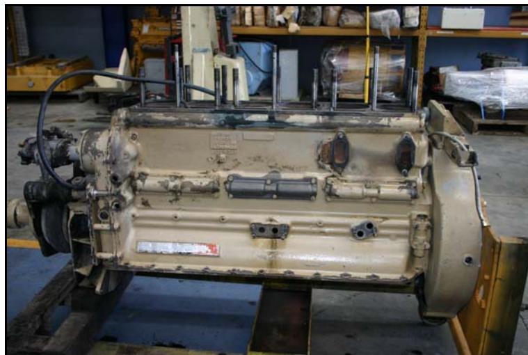
Figure 8 Underside of engine after cleaning
