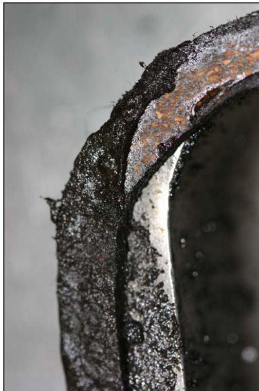
Figure 14 Witness marks of lower gasket on centre rocker cover
