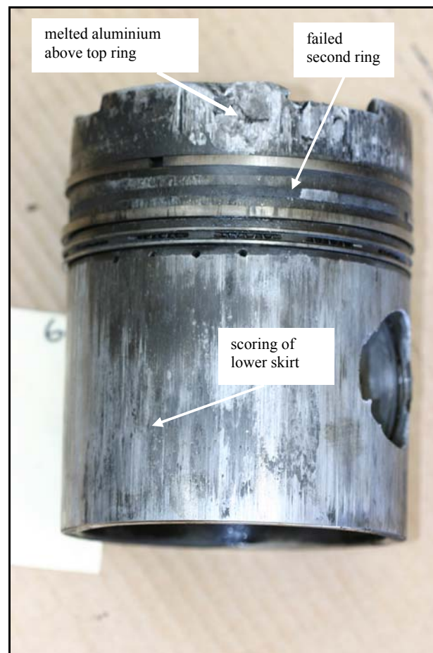
Figure 18 Scoring on No. 6 piston skirt
