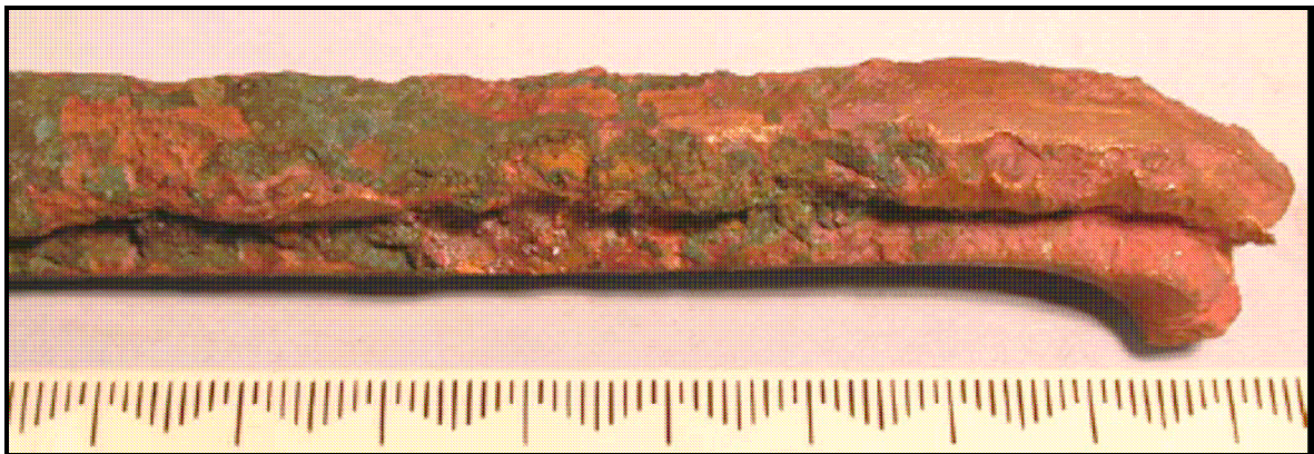
Figure 5 Deformation and degradation of contact wire labelled Sample B
