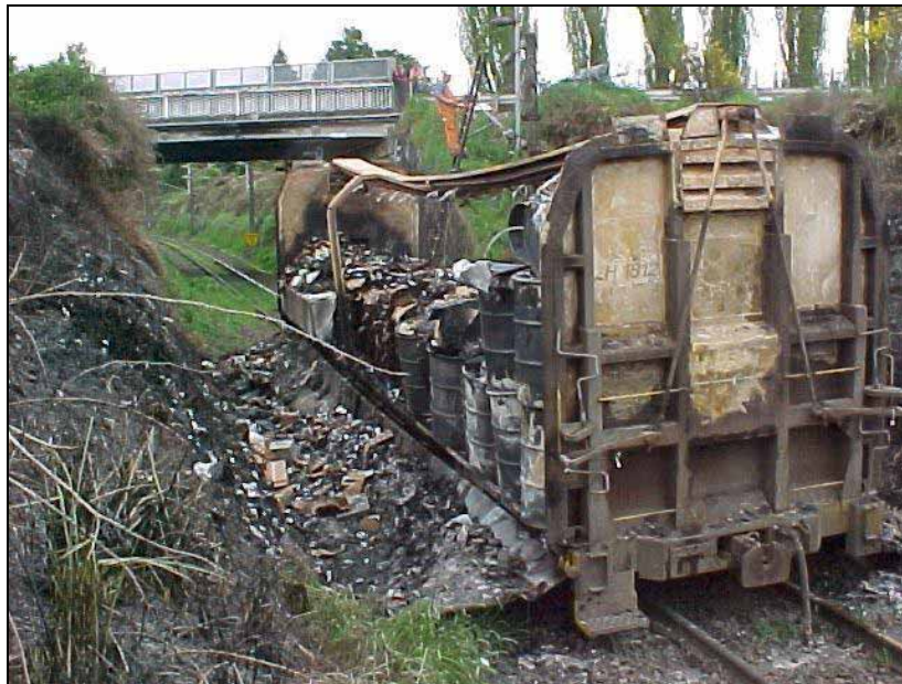
Figure 2 Fire-damaged wagon ZH1812 near Bridge 191 NIMT
