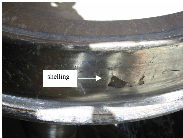
Figure 8 Shelling on the wheel tread
