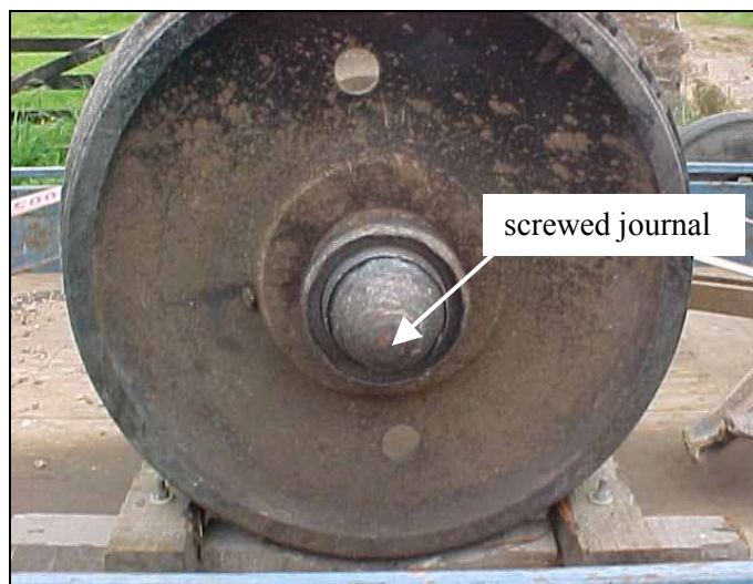
Figure 4 Recovered wheelset with failed journal
