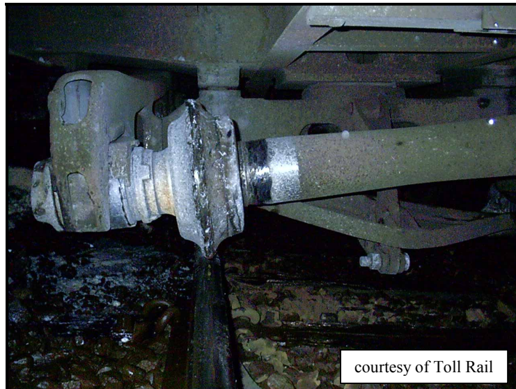
Figure 9 Derailed wheelset on wagon ZH865
