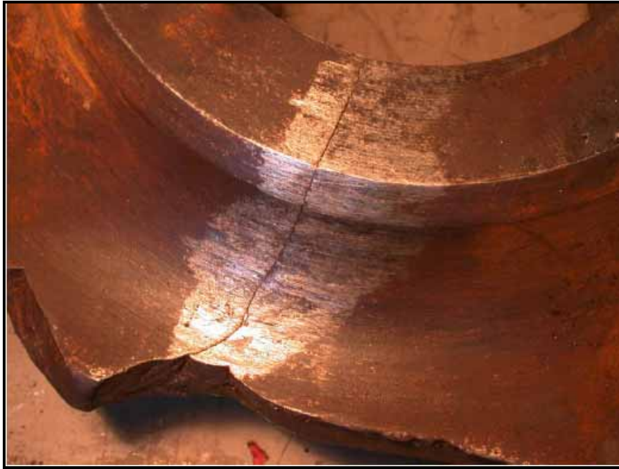
Figure 6 Crack in hub boss meeting the circumferential crack from the rim
