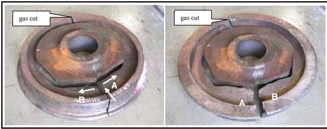
Figure 2 View of both sides of the fractured wheel
