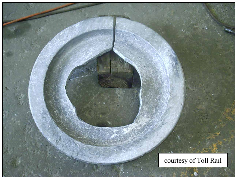
Figure 8 Outer portion of failed wheel on ZH1236
