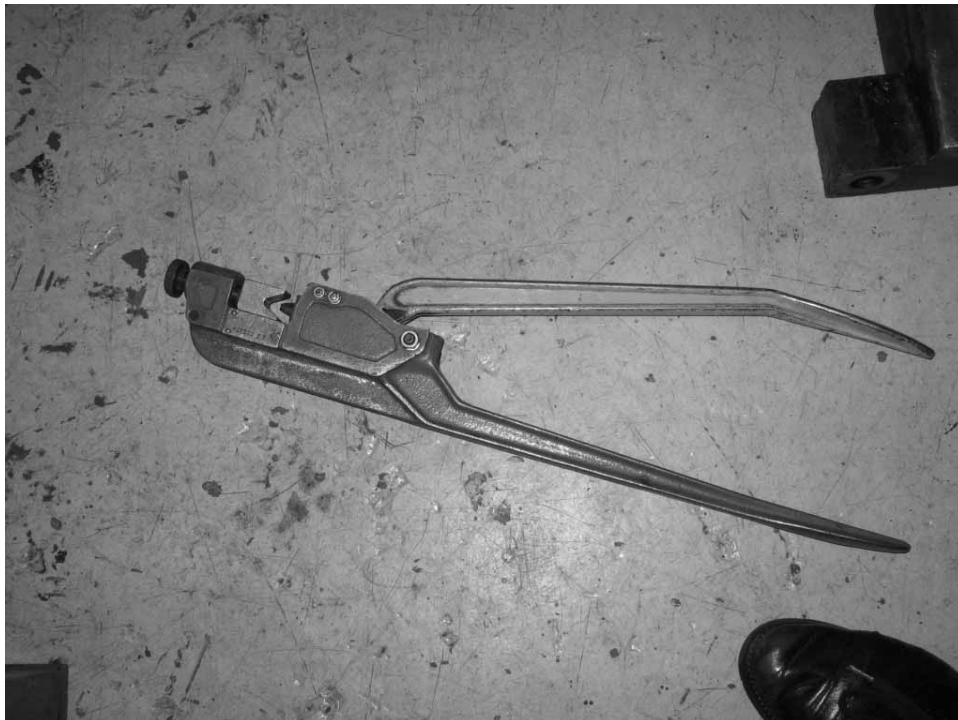
Figure 8 The manually operated, adjustable crimping tool in use at Alstom Hutt
