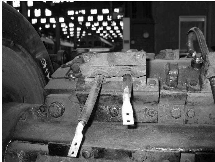
Figure 6 A 50 mm 2 lug crimped to the 35 mm 2 cable end
