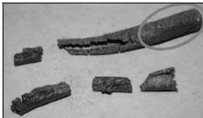
Figure 7 Remains of the internal polymer tube
