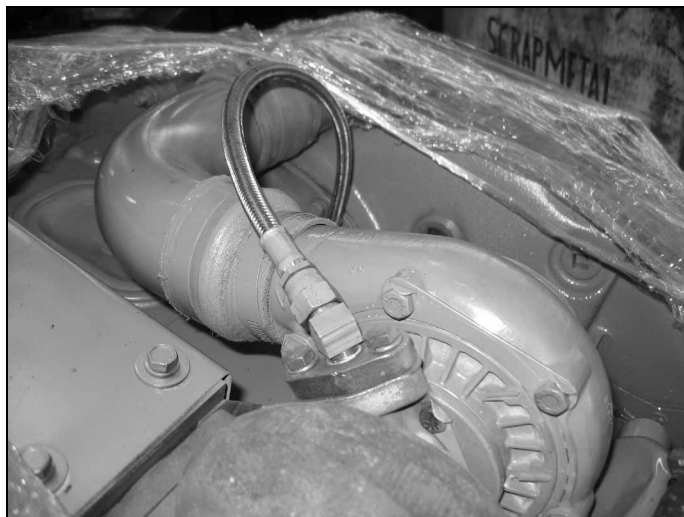
Figure 8 The new standardised fitting for the oil inlet hose
