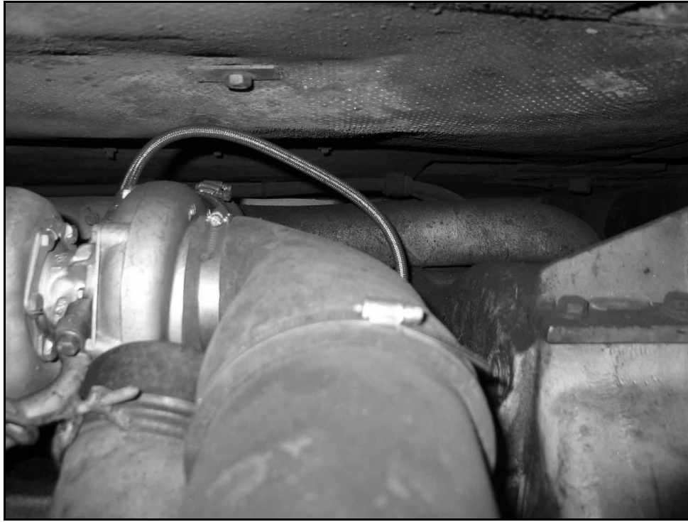
Figure 3 The replacement oil inlet hose looped over the turbocharger air inlet
