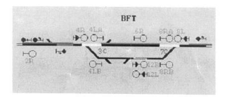
In this instance blocking has been applied on the main line. If, for operational reasons, a train needs to get to the loop, and there is still a gang active on the main line, the following can be done:
