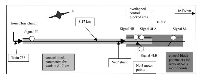
Figure 2 Christchurch-Belfast section showing the overlapped control blocked area (not to scale)
