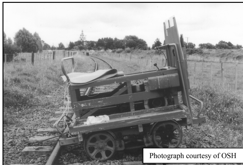
Figure 4 The derailed motor trolley at the point of derailment, looking back towards Lepperton
