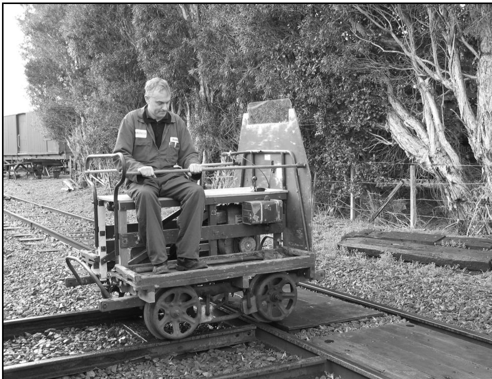
Figure 12 The restraint / handrails fitted to the motor trolley
