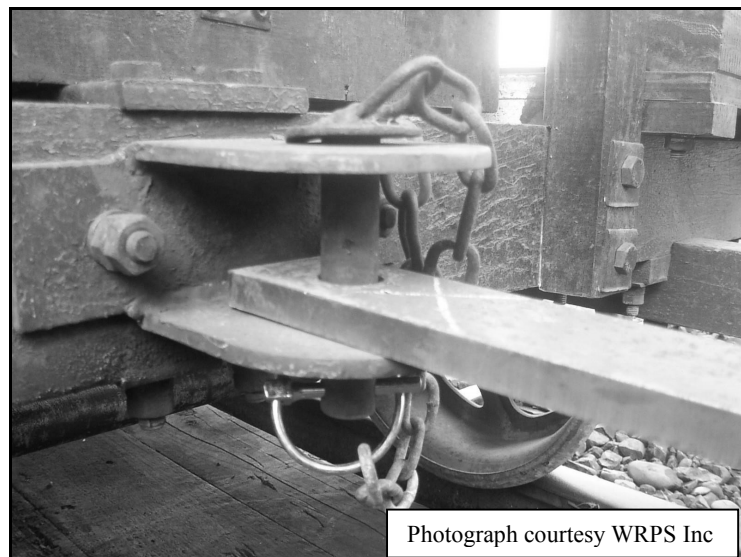
Figure 9 The new attachments for the draw gear
