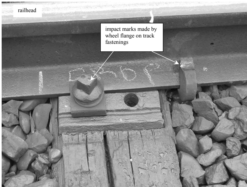
Figure 2 The point at which the wheel dropped from the railhead
