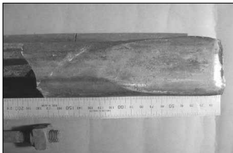
Figure 4 Vertical deformation on the new rail at the failed joint
