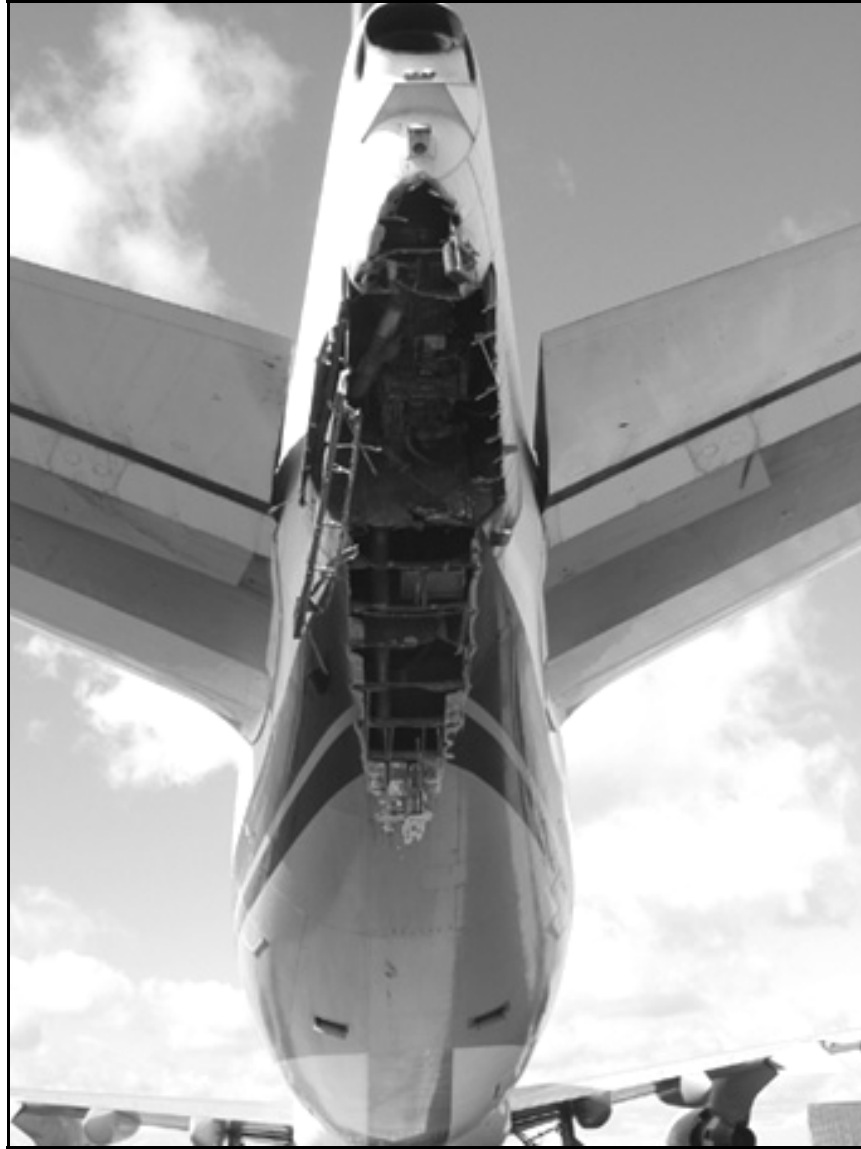
Figure 4 9V-SMT damaged tail section
