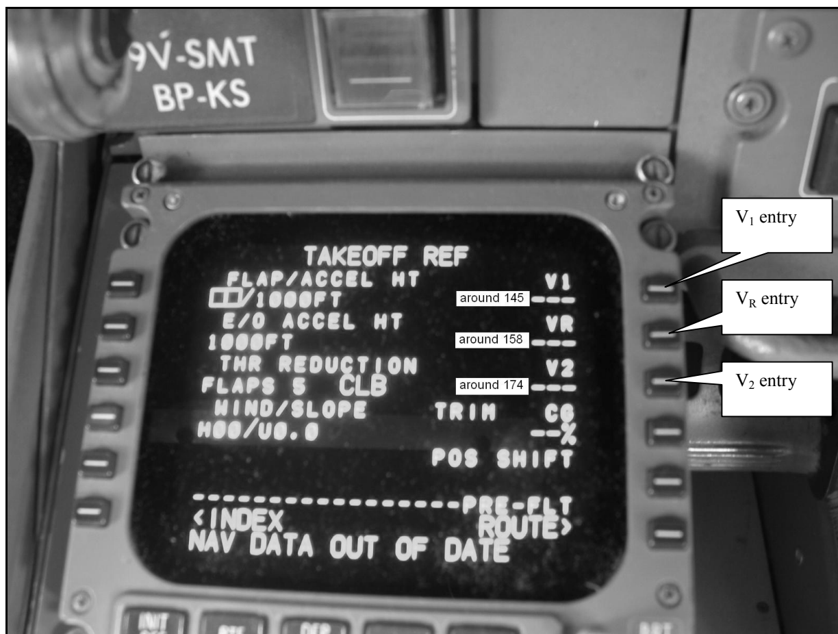
Figure 3 9V-SMT FMC display of V speeds
