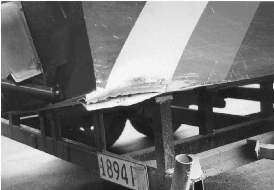
Figure 4 Damage to chine at right rear
