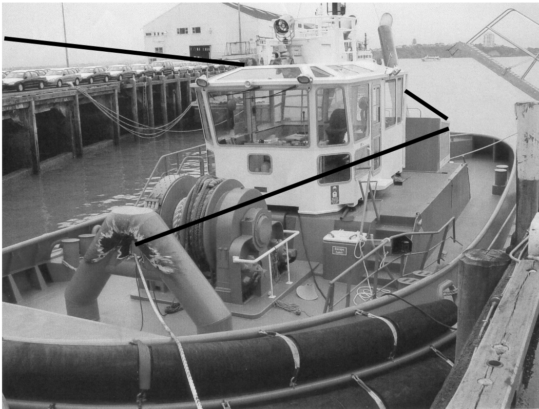
Figure 2 Waka Kume showing direction of towline and damage to port side
