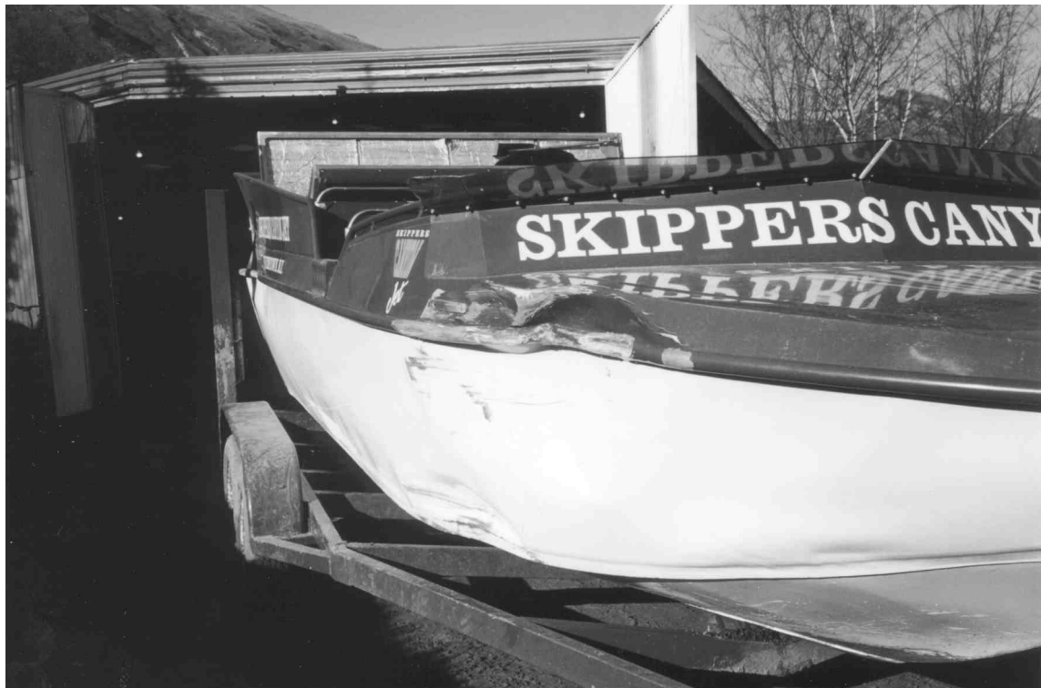
Figure 5 Damage to the starboard side of the Discovery
