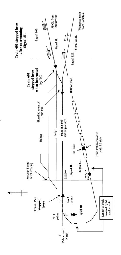
Figure 1 Woodville track layout (not to scale)
